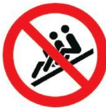
Figure K.2 - Descending in a chain is prohibited.
