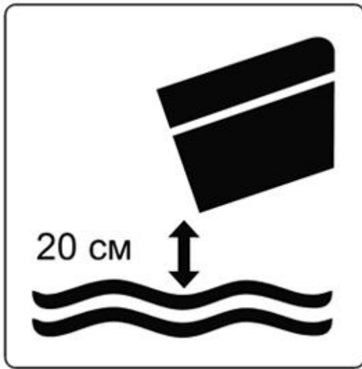
Figure L.3 - Drop Height into the Water at the End of the Descent
